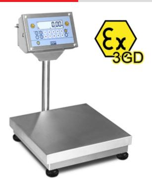
Fully stainless steel bench scales, for specific use in <u>ATEX</u> hazardous areas. Powered by a long lasting rechargeable battery which allows an easier installation directly where it's needed. These scales don't need a power supply socket in dangerous zone nor ATEX proof power supply cables. Provided with ATEX declaration of conformity. Ex II 3GD IIC T6 T130°C X protection.
